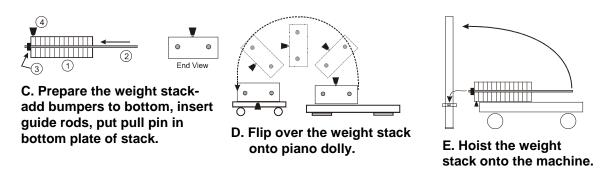
Figure 10. Putting on the weight stacks.
